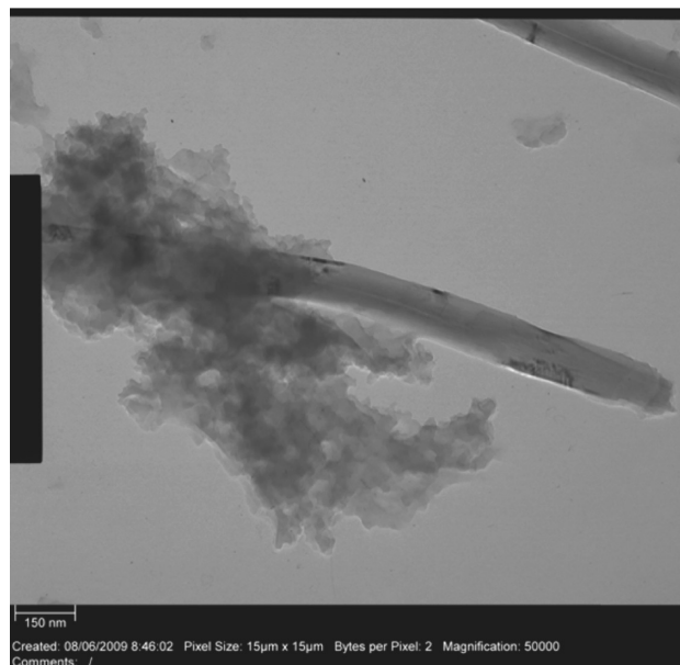
Figure 7. TEM micrograph of MWCNT-CW b -DES. Bar is 150 nm.
